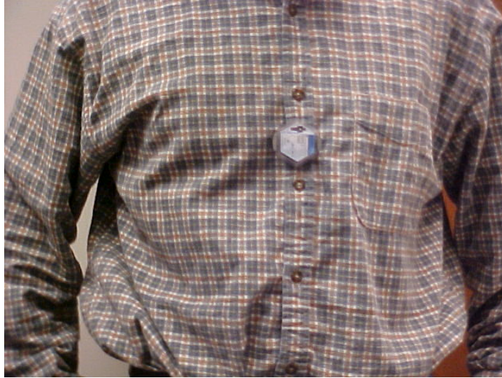
Figure 1. The whole-body dosimeter should be worn in the upper torso area between the waist and neck
