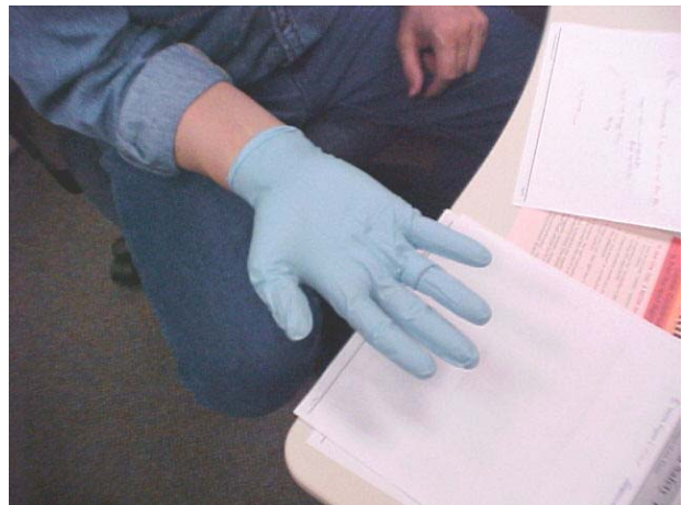
Figure 2. The ring dosimeter should be worn on the index, middle, or ring finger of the dominant hand (hand most used during radioactive work). The ring should be turned so the label faces the source of radiation, and worn inside the gloves.
