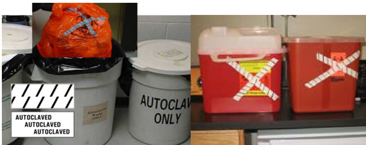
Figure 1 Autoclave tape utilizes a chemical reaction to indicate a temperature of greater than 121°C was achieved. This color change is usually displayed with hash marks or words that appear on the tape when proper temperature is reached.
