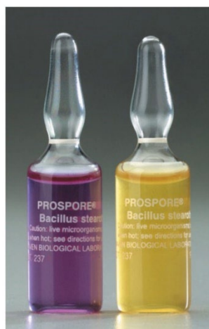
Figure 3 Color change indication for spore growth. No growth is indicated by purple color (left), growth is indicated by color change to yellow and increased turbidity (cloudiness) (right).
