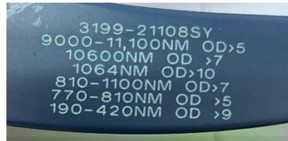
*OD Markings on Laser Safety Eyewear for Different Emitted Wavelengths*
