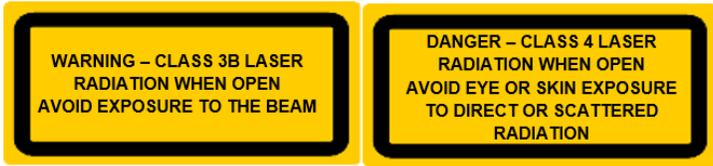
*Sample Service Panel Laser Hazard Signs Requiring a Special Tool*
