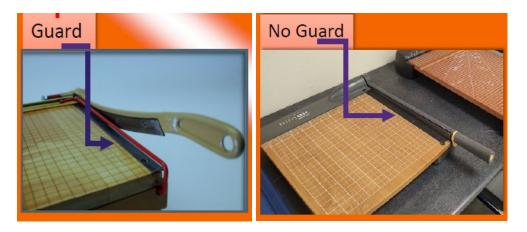
At another university in the United States, an incident occurred recently involving a cutter without a guard. A staff member cut the tip of their finger off using a manual paper cutter while cutting index cards for a class. The paper cutter did not have a finger guard on it. The staff member is currently healing fine from this amputation.
