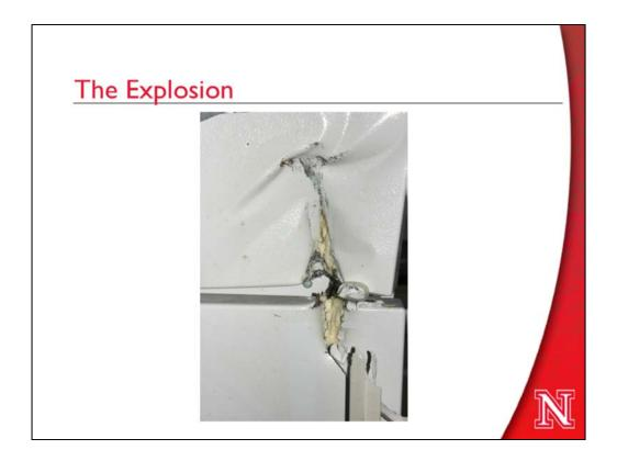
Damage to the refrigerator where part of the tank hit it.
