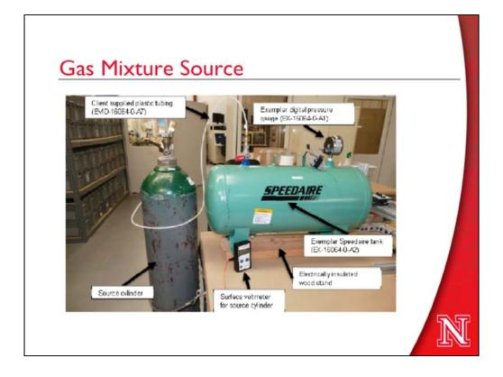
A postdoc researcher purchased a 50-liter, low pressure tank, installed a pressure gauge, and a ball valve so that hydrogen, oxygen, and carbon dioxide could be transferred from compressed gas cylinders into the tank. The tank is then connected to the bioreactor and the gas mixture slowly sparged through it.
