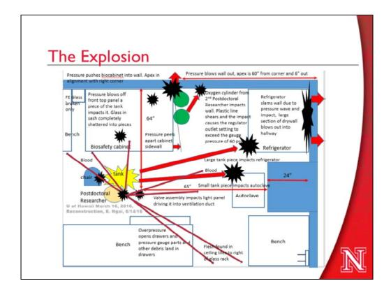
Start with the postdoc and moving clockwise around the image, see the damage done to the lab.
