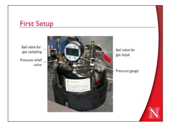
This is a growth chamber. Petri dishes with the bacteria, etc., are placed inside.
