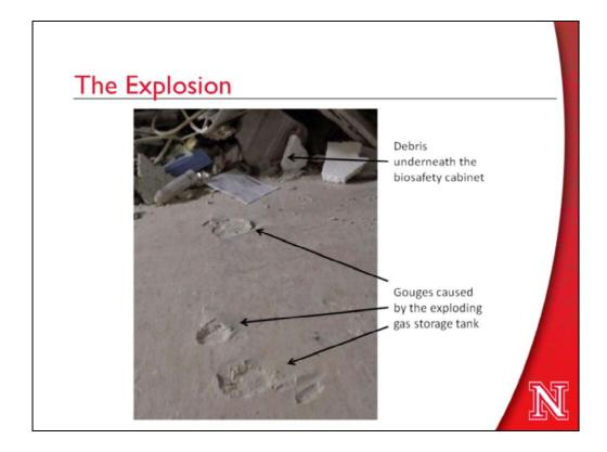
Gouges in the floor from the tank legs.
