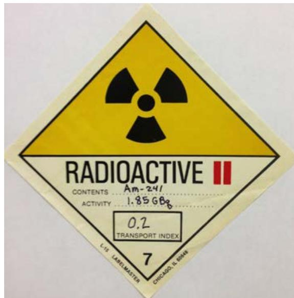
8. Required markings on the transportation cases for the **Troxler (Models 4301 and 4302)** gauges are:
