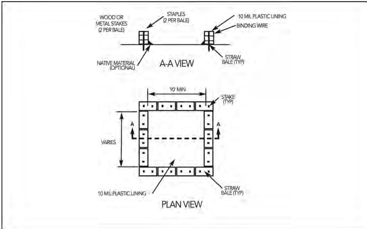
**Figure 9-63 Installation of Above Grade Washout Facility**
