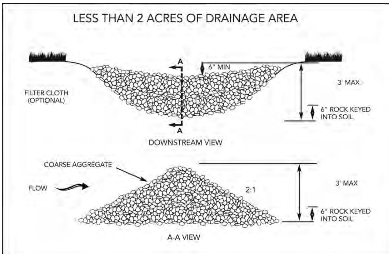
Figure 9-15 Rock Check Dam – Less Than 2 Ac.
