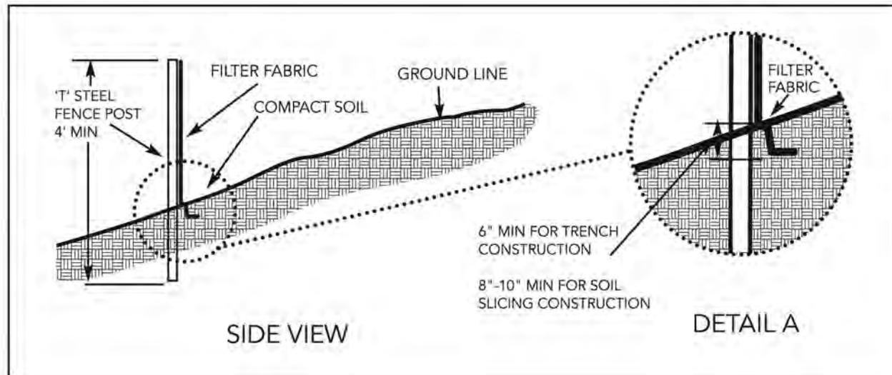
Figure 9-5 Typical Section of Silt Fence Installation
