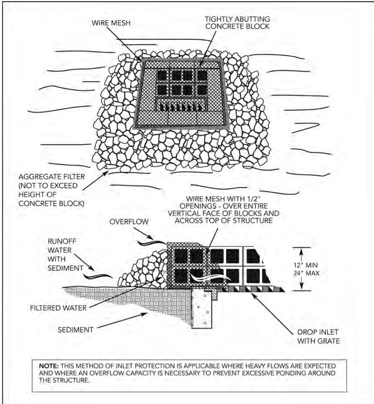
Figure 9-8 Block and Aggregate Drop Inlet Sediment Filter
