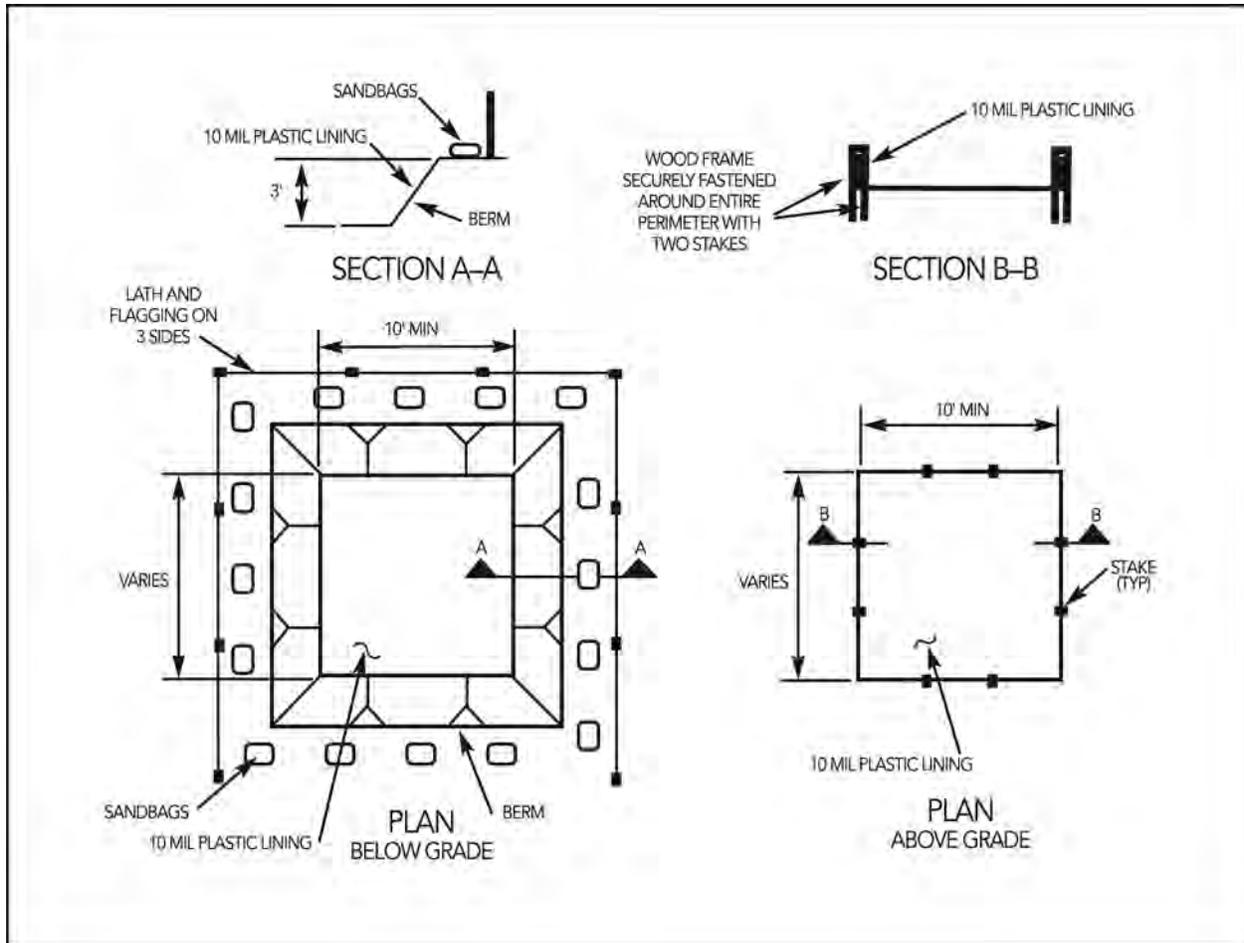
Figure 9-62 Installation of Below Grade Washout Facility
