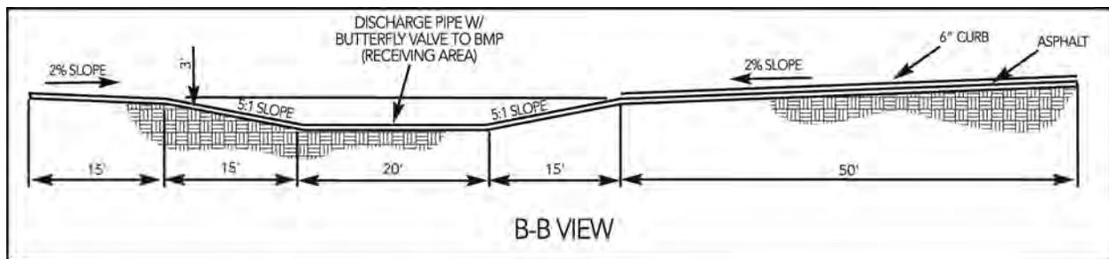
Figure 9-56 Wheel Wash Elevation View (Section B-B)
