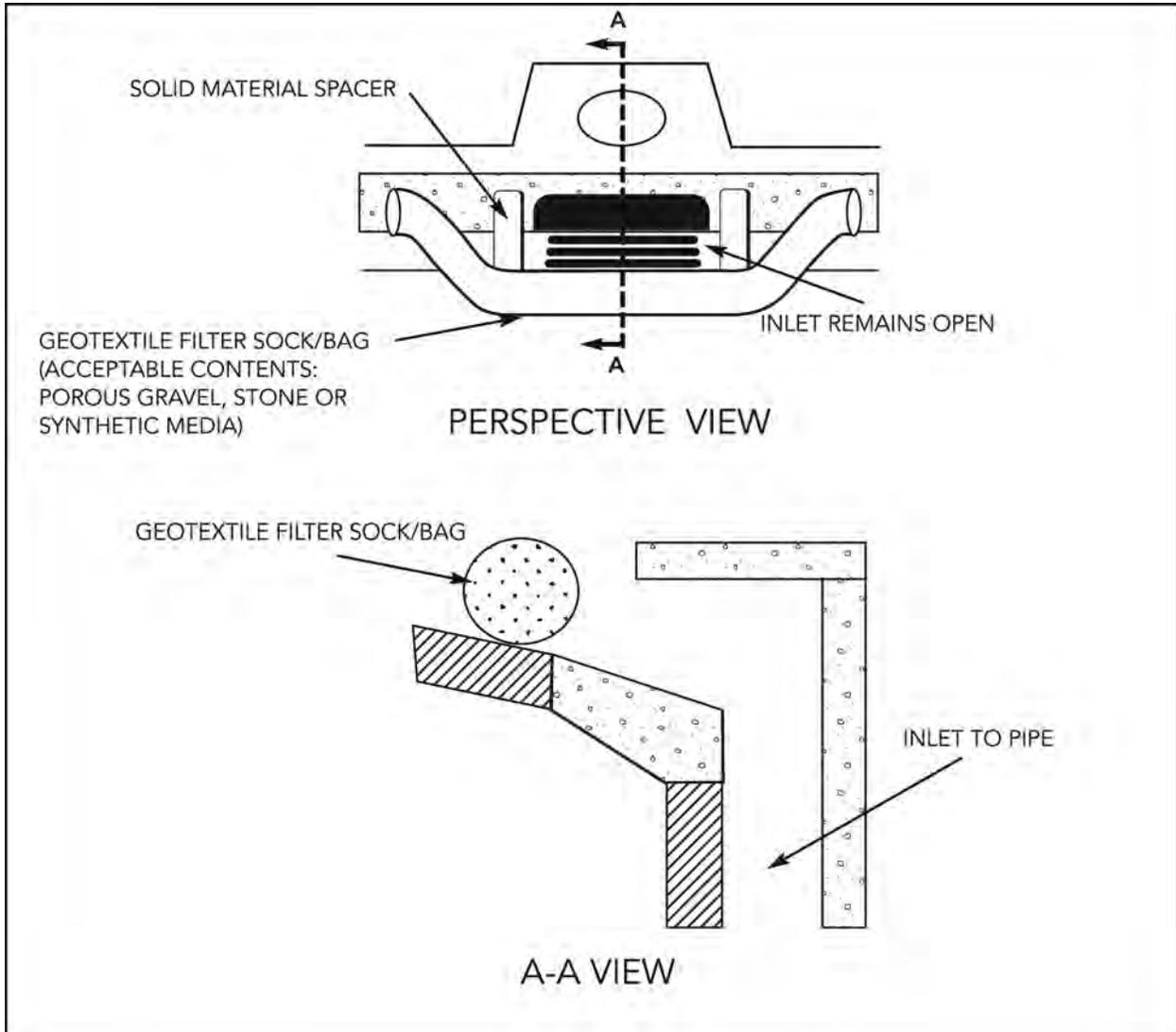
Figure 9-10 Curb Inlet Protection With Filter Sock
