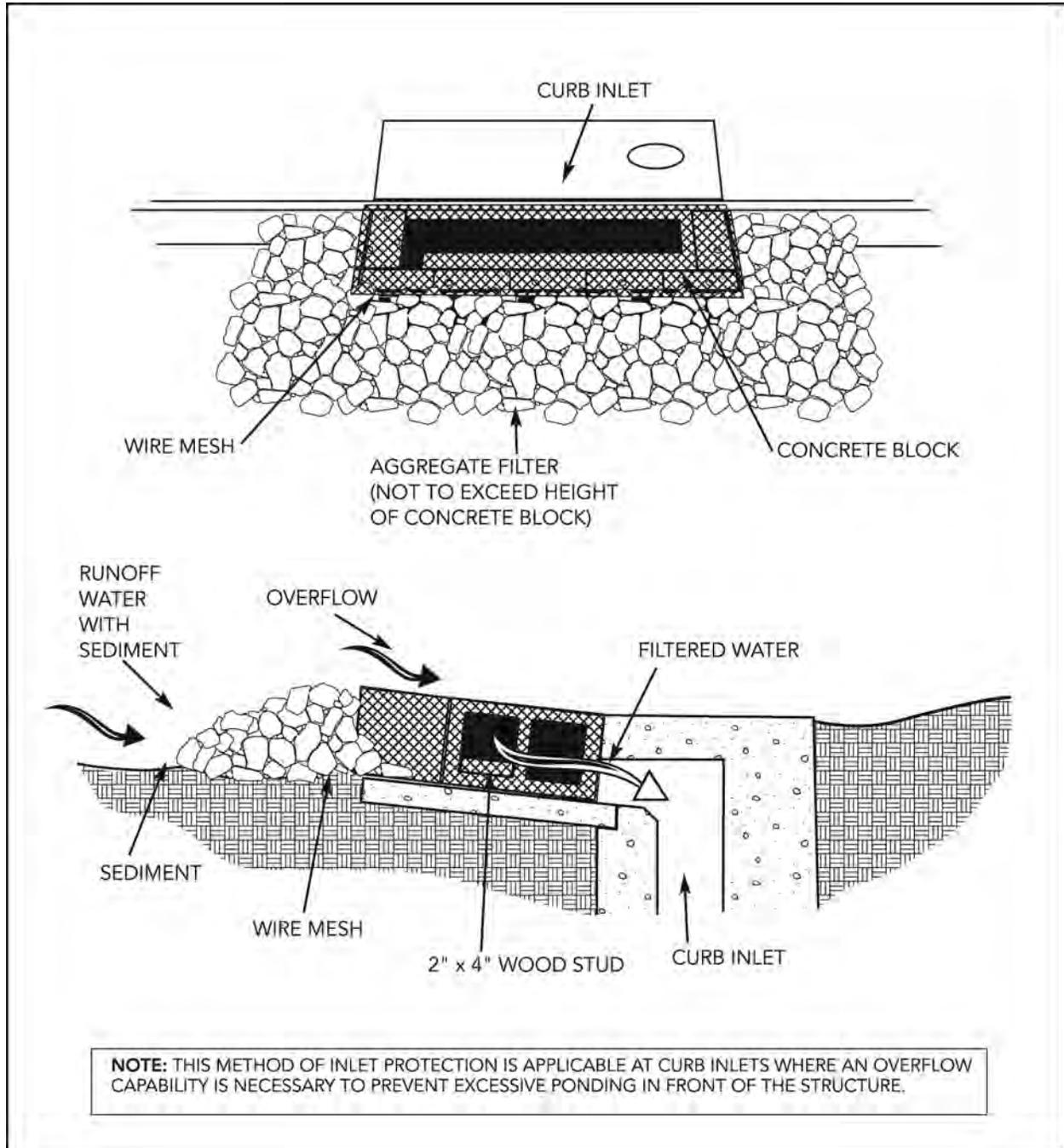
Figure 9-9 Block and Aggregate Curb Inlet Sediment Filter
