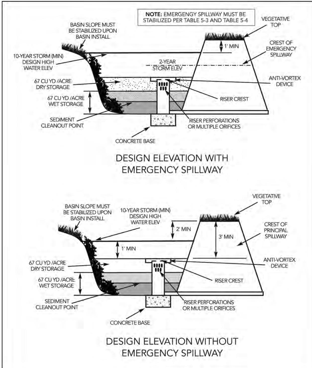
Figure 9-30 Design Elevation for Temporary Sediment Basin
