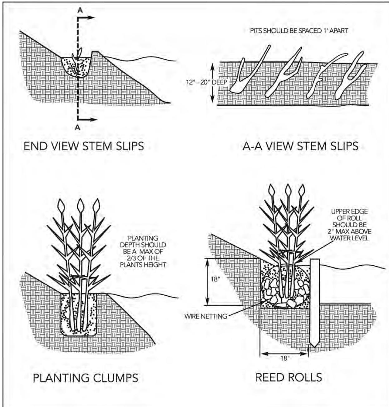
Figure 9-42 Methods of Establishing Reed Bank Vegetation
