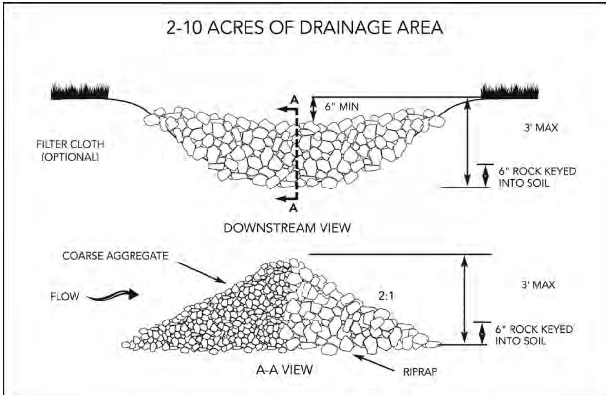
Figure 9-16 Rock Check Dam – 2-10 Ac.
