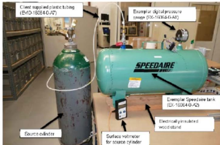
A postdoc researcher purchased a 50-liter, low pressure tank, installed a pressure gauge, and a ball valve so that hydrogen, oxygen, and carbon dioxide could be transferred from compressed gas cylinders into the tank. The tank is then connected to the bioreactor and the gas mixture slowly sparged through it.
