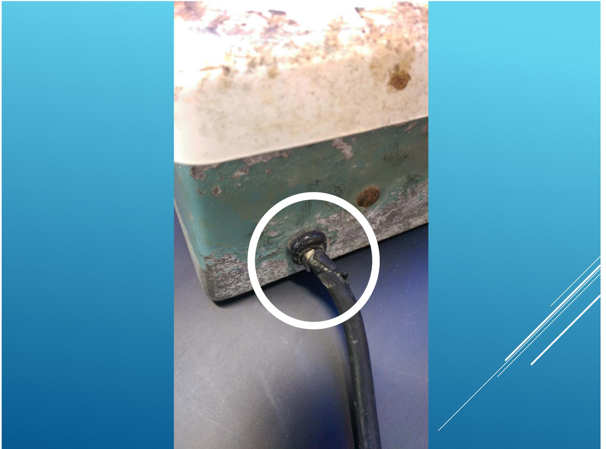
Section 1926.416(e)(1) provides that "worn or frayed electrical cords or cables shall not be used." Superficial nicks or abrasions — those that only slightly penetrate the outer jacket of a flexible cord, and do not permit the cord to bend more in that area than in the rest of the cord — do not normally render a cord "worn or frayed." Therefore, there is no need to repair or replace such a cord.
