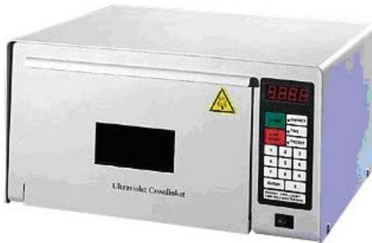
**UV Crosslinker** - Used to attach nucleic acids to a surface or membrane following blotting procedures. Crosslinkers are equipped with door safety interlocks, which similar to a household microwave, prevent operation of the machine when the door is open. If the interlock system is not functioning correctly, refrain from using the device and contact the manufacturer.
